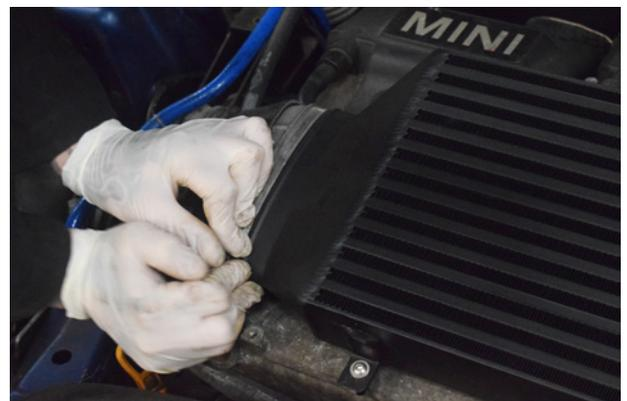
16. Manipulate the intercooler in to position on the hot side.
