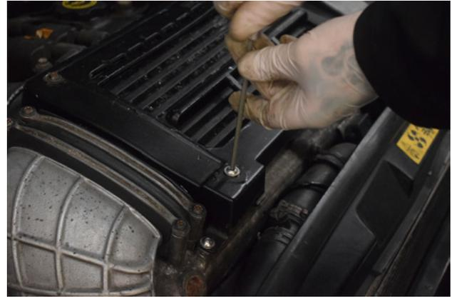
2. Remove 4X T30 screws securing the intercooler cover.
