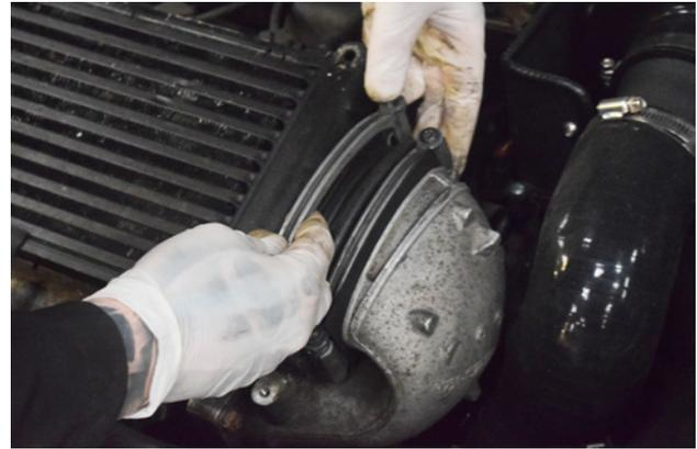
10. With the screws removed, the C clamps can be removed or left loose until the intercooler is out.
