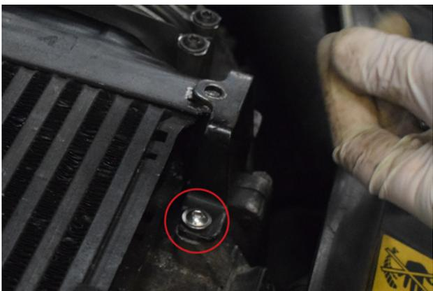
5. Remove 4x T30 screws on the factory intercooler support brackets.
