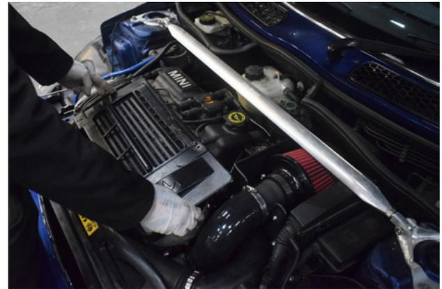
4. Once all four T30's have been removed you can lift off the cover.
