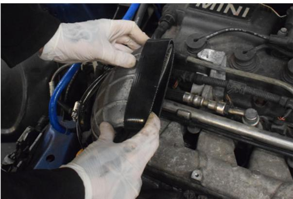
17. Push silicone joint over the hot side hard pipe.
