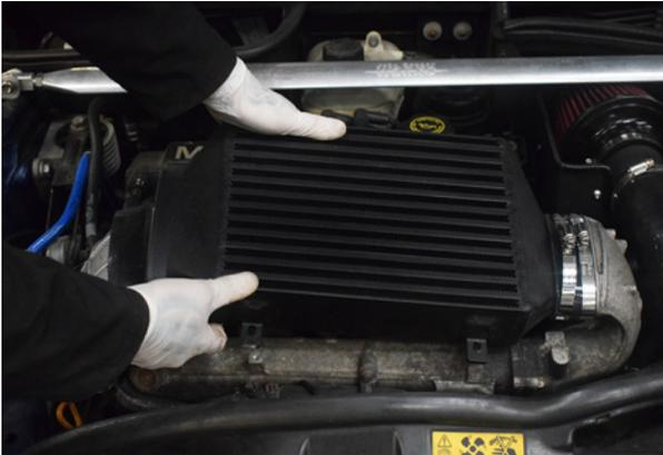
13. The intercooler needs to be pushed into the cold side joiner/hardpipe first.
