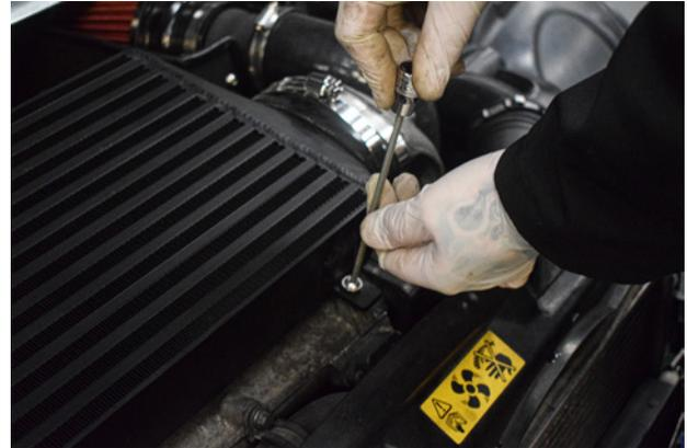
14. Use supplied hardware to secure the intercooler brackets.
