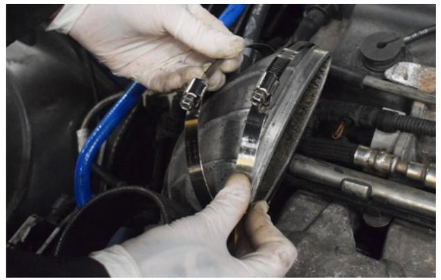
16. Slide the clips over the hot side hard pipe.
