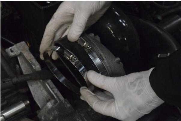
15. Slide the supplied silicone and clips over the cold side hard pipe.
