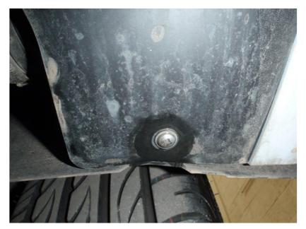
**3.** Looking under the car up at the arch liner there is a pozidriv/Phillips screw, undo this on both sides of the vehicle.
