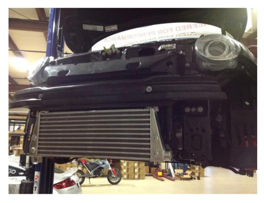
Using the long bolts and penny washers provided, bolt the intercooler to the crash bar as shown
