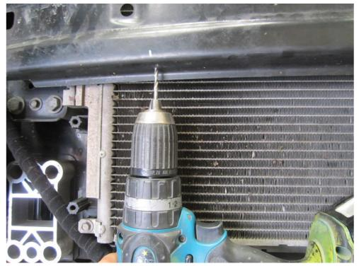
**23.** Fix the intercooler into position using the two M8 x 16 hex heads provided ensuring the penny washers and sprung washers are also used as pictured below.
