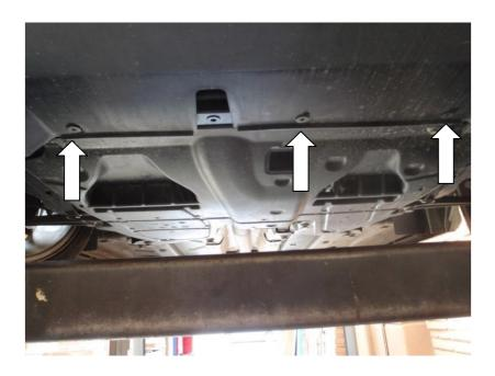
**5.** Undo the three T30 screws holding the bumper to the chassis.
