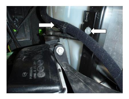
**15.**Undo the clip holding the washer bottle pipe and undo the 10mm bolt on the driver's side, you will now be able to remove the complete intercooler unit by pulling upwards with an even force to release the bottom pegs from the rubber grommets.
