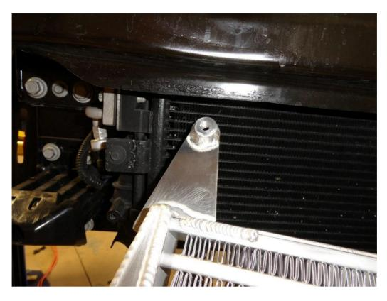
**18.** FOR U.S. CUSTOMERS AND INTERCOOLERS SUPPLIED WITHOUT A LOWER CRASH BAR: Push the mounting tabs on the intercooler up behind the crash bar so that the bosses on the ends line up with the holes already in the crash bar.
