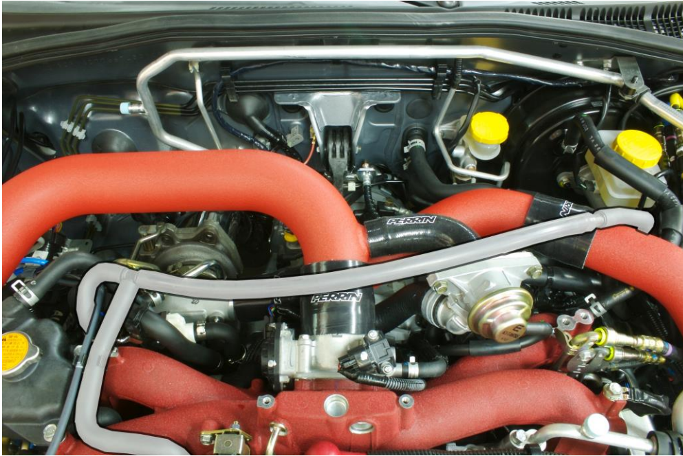
1/2" Fuel Hose, and Connectors Highlighted to Show Routing
