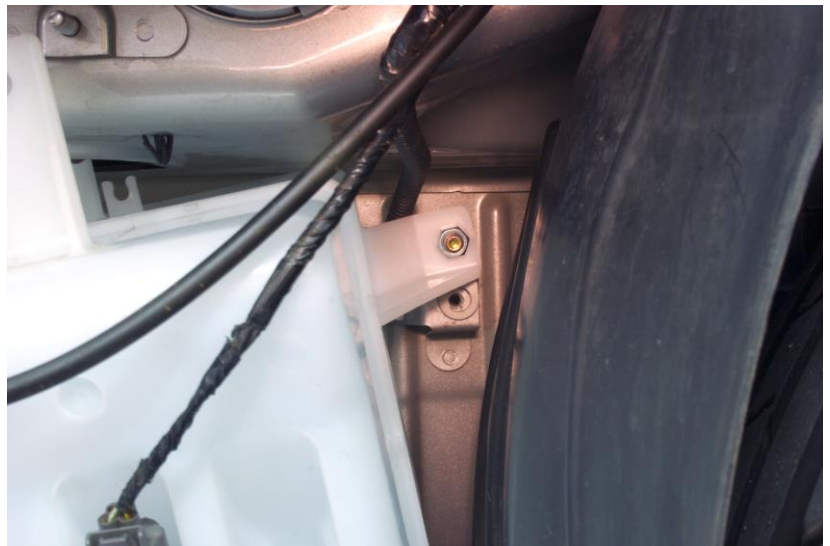
Washer Bottle Mount Being Offset by Bracket
