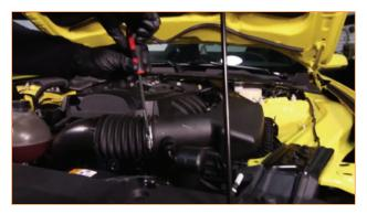
**2.** Disconnect the plug from the intake air temperature (IAT) sensor.
