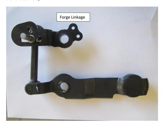
10. You are now able to fit the Forge linkage to the gearbox, fit the dual linkage first leaving the small single linkage to last. This bit is a bit fiddly to do but with patience it will fit perfectly. DO NOT FORCE THE LINKAGE ON TO THE GEAR BOX. The toothed splines are keyed and will only fit on in one orientation. ON VELOSTER N YOU MAY NEED TO ADJUST THE CABLE END TO SHORTEN THE CABLE.
