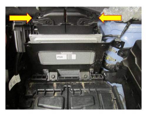
3. Once unplugged you can now remove the three 10mm fasteners that hold the ECU in position, two at the bottom and one at the top right. Use some long nose plyers to remove the plastic fastener that is holding the negative battery cable to the ECU bracket.
