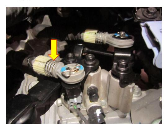
11. Tighten the three fasteners that hold the linkage to the gearbox, then test to see how the shift feels inside the car. If you think it needs adjustment this is the time to do so, now reassemble by following the steps 1-6 in reverse.
